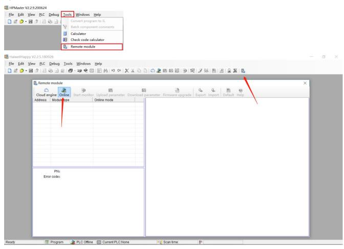
The default address of the Module is 1 with format 19200, N 82 RTU, and the online success is as follows:
