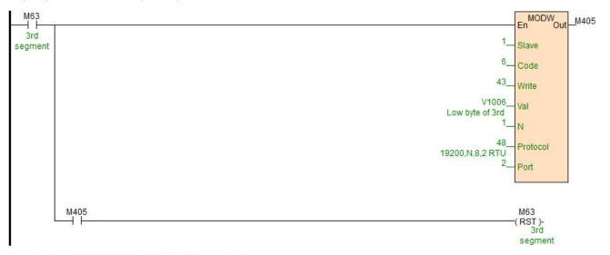
//Network 6 Step6: Write "2" into CR26H to end calibration.
