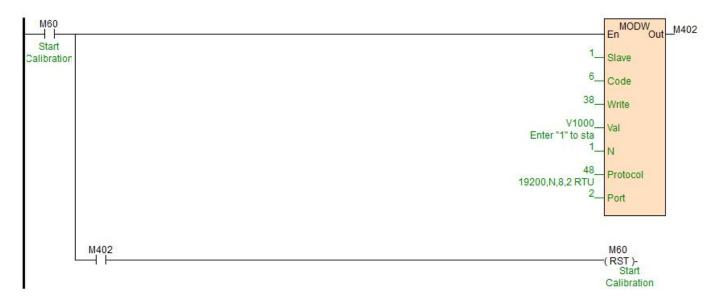
//Network 3 Step3: In the first segment of calibration, put a standard weight on the pan connected to the load cell module. The weight of the counterweight should be written into CR27H(16 bits) You could continue to step 6 if multiple segments of calibration are unnecessary.
