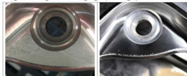
Overcut and chatter marks at corner
