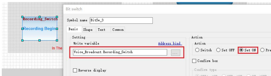
Figure18 Recording Switch Bit Switch
